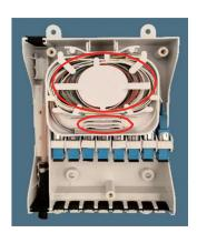
5. Close the cover, plug outgoing pigtails through sealing rubber.
