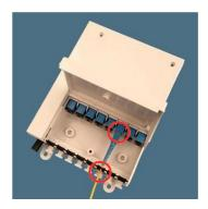
6. Install the box with expansion screws and finish the installation.
