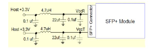
**Recommended Host Board Power Supply Circuit**
