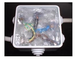
Cover the connection completely with SOFT GUM by pressing it so as to distribute the product uniformly in the box. Close the junction box.
